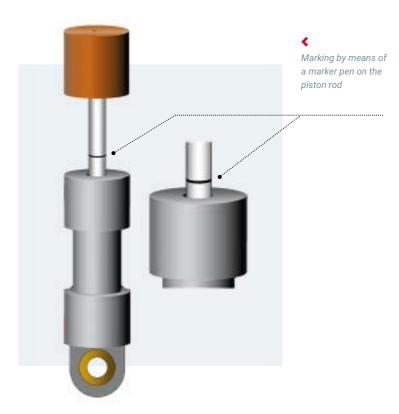
If a lowering brake valve in the hydraulic system has to be adjusted in the installed state, a number of factors must be observed before the valves are adjusted (source: technical information from SUN-Hydraulik).
