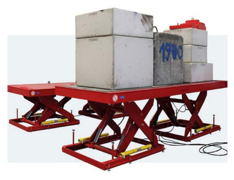
Sample application: scissors lift table from Janzen-Lifttechnik. The lowering brake valve is already integrated and preset in the cylinder connection (on the piston side)!
