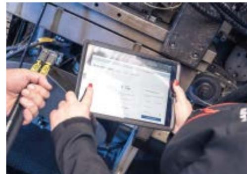
To call up all the information on the individual hose line, it is sufficient to read the label or scan the QR code using the X-CODE Manager app.
